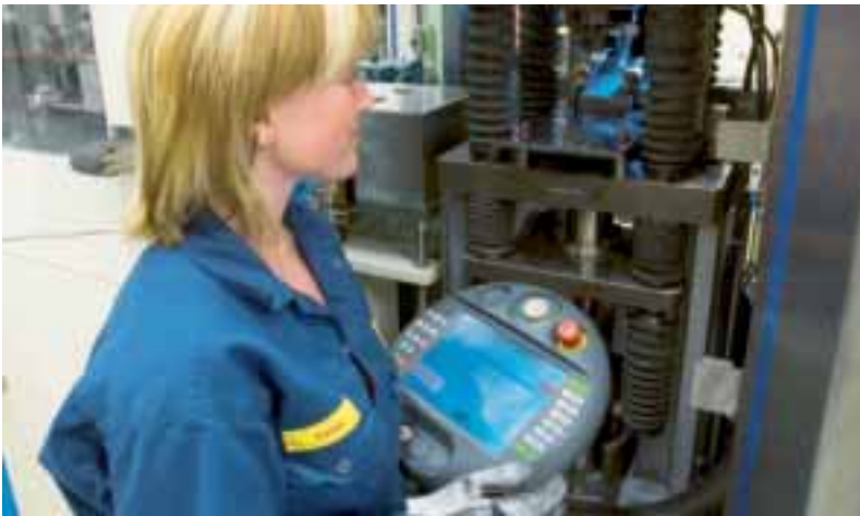
Pressing of cemented carbide tools for metalcutting applications at Sandvik's plant in Gimo, Sweden.
