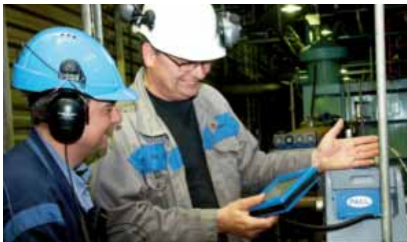
Service staff from Indutrade measure the cleanliness of filters used in the hydraulic and lubrication oil system at a paper mill.
