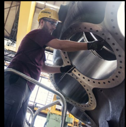
Plunge milling when machining turbine housings reduces the customer's processing time, costs and environmental impact.
